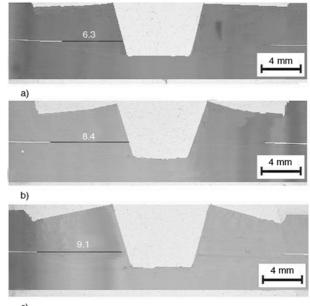
**Figure 15.** The effect of the shoulder angle on the joint cross section, (a) 1.5° shoulder angle tool, (b) 6° shoulder angle tool and (c) 12° shoulder angle tool
