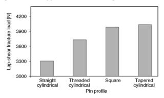
Figure 5. Lap shear fracture loads of different pin profiles
