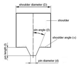
Figure 3. FSSW tool design showing geometric parameters
