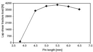
**Figure 10.** The effect of the pin length on the lap-shear fracture load
