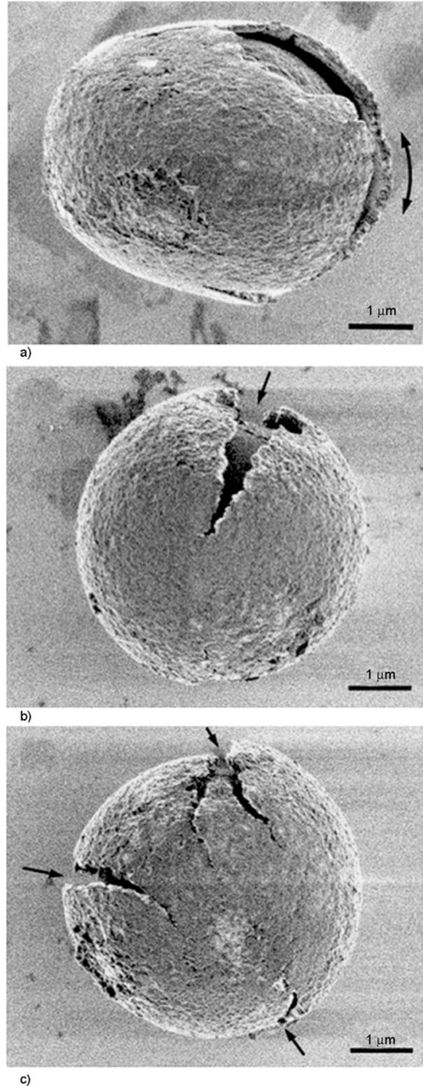
**Figure 2.** The corresponding SEM images of particles after compression at loading rate (a)  $0.02 \text{ mN}\cdot\text{s}^{-1}$ , (b)  $0.2 \text{ mN}\cdot\text{s}^{-1}$  and (c)  $2 \text{ mN}\cdot\text{s}^{-1}$ . The images are taken from top view (in the direction of compression). Electron high tension (EHT) = 0.5 kV; working distance ( $W_D$ ) = 2 mm.
