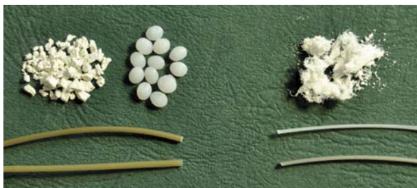
Figure 5. Compounded specimens from G 70/30 left (brownish) compared to F 70/30 (whitish) right
