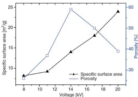
Figure 4. Specific surface area and porosity of PVDF nanofiber membrane
