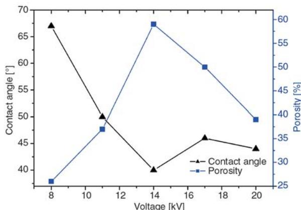
Figure 7. Diagram of the Washburn contact angle and porosity
