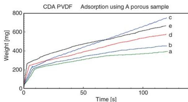
**Figure 9.** Dynamic water adsorption of the membrane electrospun with (a) 8 kV (b) 11 kV (c) 14 kV (d) 17 kV and (e) 20 kV
