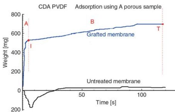
Figure 8. Dynamic water adsorption of PVDF membrane before and after acrylic acid grafting
