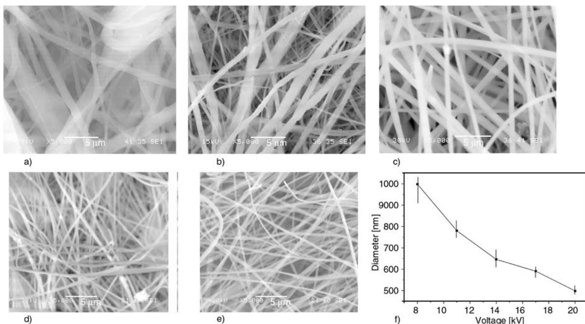
**Figure 2.** SEM images of PVDF membranes prepared with voltage of (a) 8 kV, (b) 11 kV, (c) 14 kV, (d) 17 kV, (e) 20 kV and (f) curve of diameter with voltage
