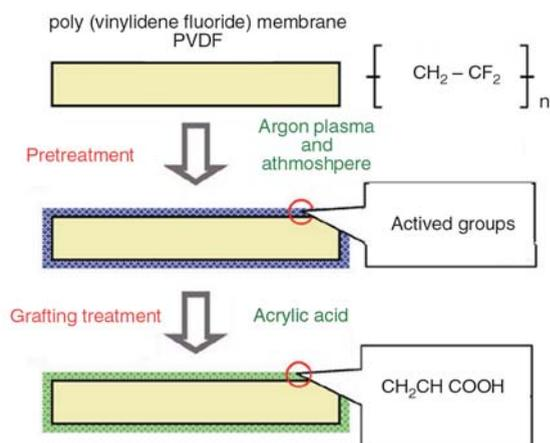
**Figure 1.** Schematic diagram of pretreatment and grafting on PVDF nanofiber membrane
