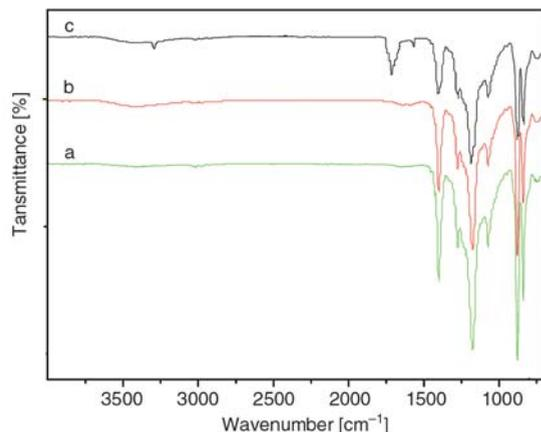
**Figure 3.** FTIR spectrum of (a) original PVDF membrane, (b) plasma treated PVDF membrane and (c) grafted PVDF membrane
