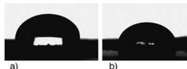
Figure 5. Micrograph of surface contact angle of (a) untreated membrane (b) membrane grafted with acrylic acid
