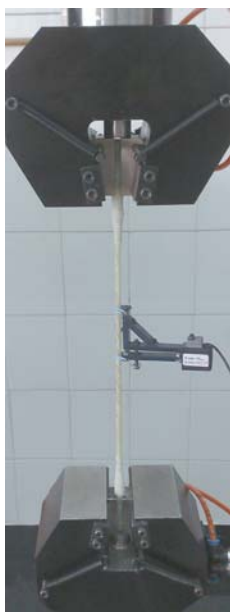
Figure 6. A specimen during tensile test
