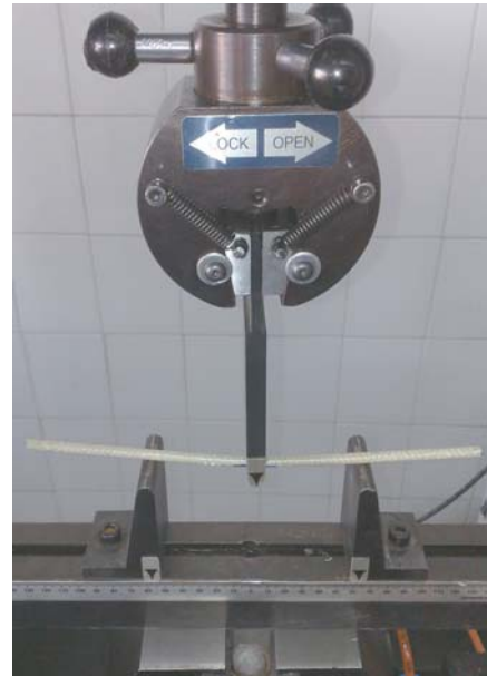
Figure 7. A specimen under bending test
