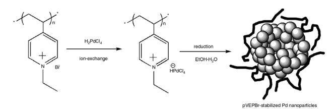
Figure 2. Formation scheme of Pd nanoparticles by using pVEPBr
