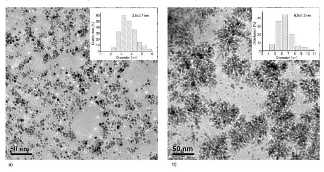
Figure 1. TEM images of pEVPBr-Pd nanoparticles before (a) and after recycling twice (b). The inset shows the particle size distribution
