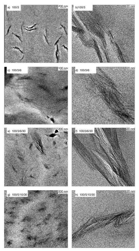
Figure 5. TEM images of PP/clay/MAPP/wood flour hybrids. a) and b) PP/clay: 100/3; c) and d) PP/clay/MAPP: 100/3/6;
