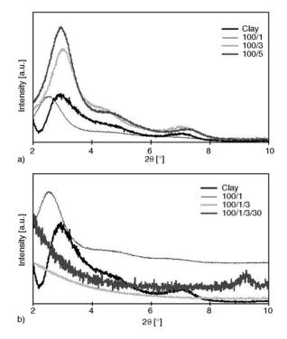
Figure 4. WAXD patterns of selected composite systems. (a) clay and PP/clay hybrids; (b) clay, PP/clay, PP/clay/MAPP, and PP/clay/MAPP/wood flour hybrids
