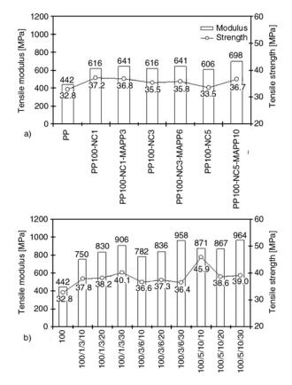
Figure 3. Tensile properties of (a) PP/clay/MAPP hybrids; (b) PP/clay/MAPP/wood flour hybrids
